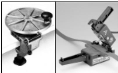
The Skiver sands the belt ends to make an overlapped joint. Once glued, the Heat Press is used for hot joining the belts after they are skived.
